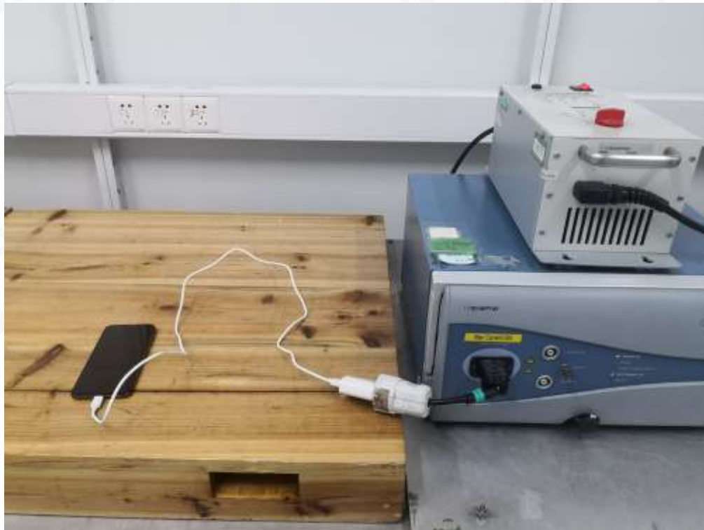
EFT SURGE and DIPS IMMUNITY TEST SETUP
