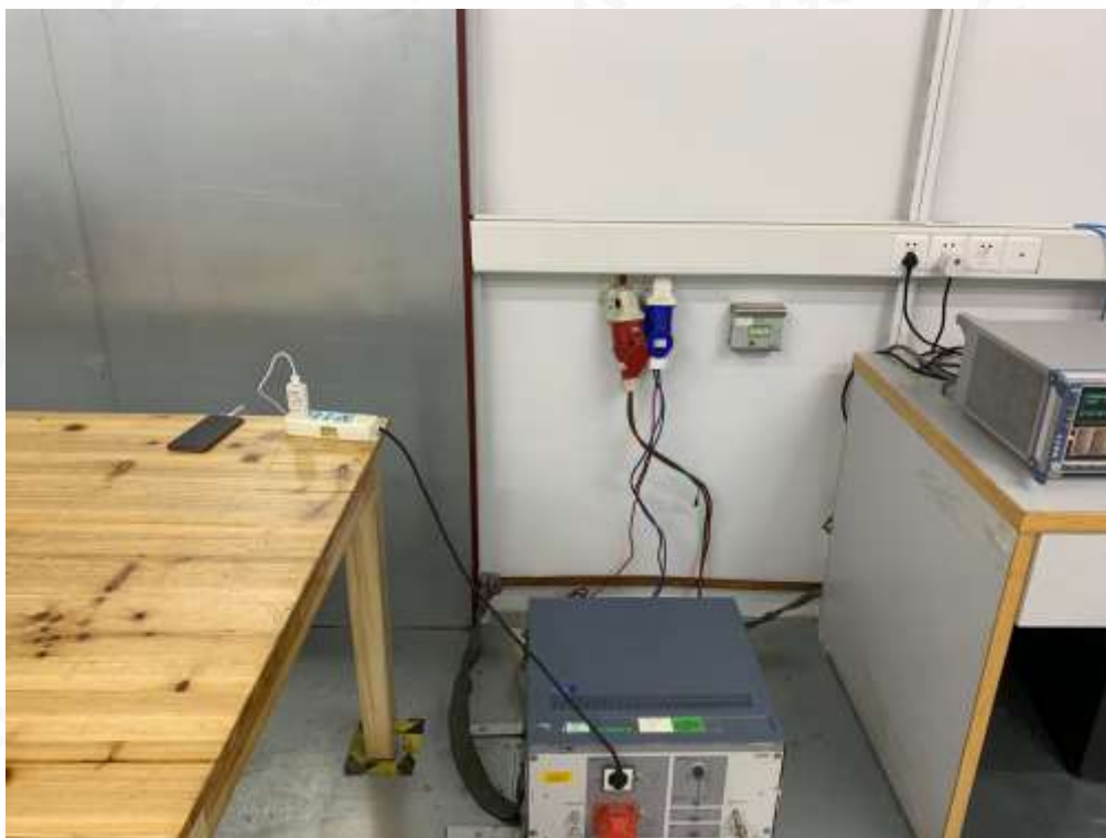
EN 55032 RADIATED EMISSION TEST SETUP
